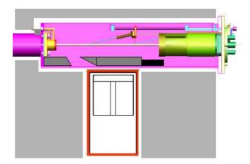
**Fig. 3.** Schematic view of the inner part of the target chamber. The internal lead collimator, the beam power calorimeter, the movable setup for the silicon detector and the long collimator before the carbon foil (at  $20^{\circ}$  with respect to the beam direction) are shown. The HpGe detector is positioned below the target chamber.
