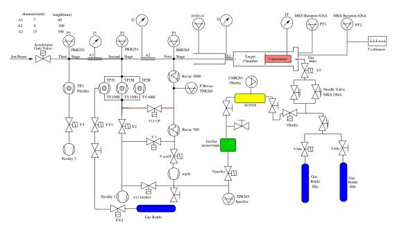
Fig. 2. Schematic diagram of the windowless gas target system.
